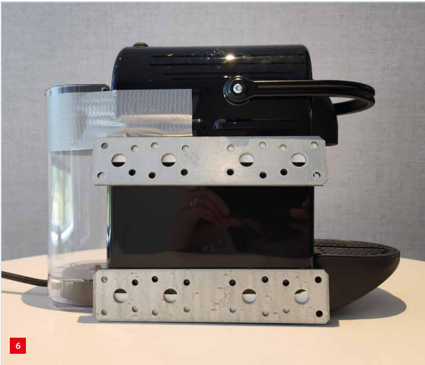
The metal strip adaptation attached to the side of the coffee machine.
